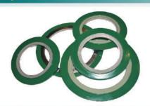
Our Spiral Wound Metallic Gaskets are skillfully manufactured by spirally winding a preformed metal strip and filler on the outer periphery of metal winding mandrels. Its winding mandrel outside diameter forms the inner diameter of the gasket and the hoop strip continually wounds until the required outer diameter is attained.
