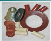
An effective form of controlling losses due to corrosion. They can be used to control stray electric currents in piping at oil, gas, water, refinery and chemical plants and increase the effectiveness of cathodic protection systems and confine or eliminate electrolytic corrosion. Most common components being a Gasket, Sleeves for bolt protection, and washers for nut protection. The variety of component materials is dependent upon application.
