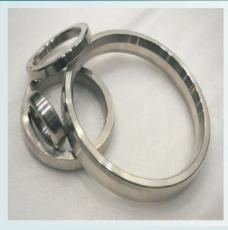
We manufacture Ring Joint Gaskets conforming to R series in Octagonal / Oval shape, Bx and Rx series of API std 6A and ASME B 16.20. They are used in the production and refining process pipelines of Oil and Gas Industries.
